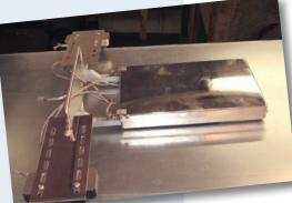
The design of the CoilPaq allows you to place this instrument on the moving coil without stopping the line.
